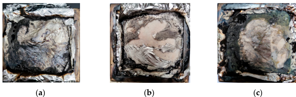
Figure 6. Images of residue after the cone calorimeter test using different materials: (a) Base asphalt, (b) epoxy resin, and (c) epoxy asphalt.
