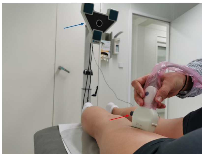
Figure 2. Ultrasound-based, three-dimensional movement analysis system. The photo shows the microphone of the device (blue arrow) and a marker (red arrow) attached to the transducer. The marker constantly sends an acoustical signal which is recorded by the microphone. As the transducer (and with this, the marker) is moved over the marked 3 cm distance on the skin, the travel time changes, which indicates probe (marker) movement.
