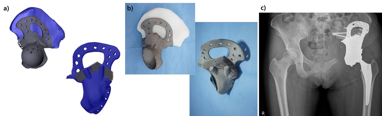
Figure 1. Pelvic implant manufactured by metal 3D printing for a 35-year-old woman who received surgery for Ewing sarcoma of the left pelvis. (a) Designs and (b) photographs revealed that the pelvic implant has both solid and lattice structures. (c) A postoperative plain radiograph of the applied pelvic implant.
