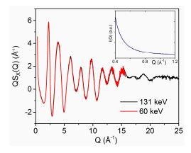
**Figure 1.** X-ray diffraction structure factors  $Q \cdot S_X(Q)$  measured on the 2015 amorphous hafnia sample obtained using incident X-ray energies of 131 keV (black) and 60 keV (red). (Inset) Small angle scattering  $(Q = 0.4-1.2 \ \text{Å}^{-1})$  measured at 60 keV (blue) and fit corresponding to the equation  $y = a + b \cdot Q^{-3.94}$  (dashed line).
