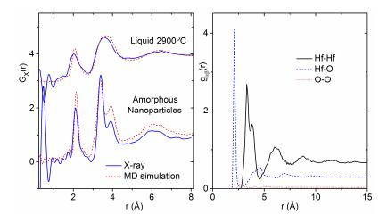
**Figure 9.** (Left) X-ray pair distribution functions of liquid  $HfO_2$  compared to the ab initio simulations performed in this study (shifted top, see text) and amorphous hafnia nanoparticles compared to the classical MD simulations performed in this study based on the parameters given by Broglia et al. [1]. (**Right**) The partial pair distribution functions for the amorphous nanoparticle simulation weighted by the Q = 0 factors for the X-ray case given in Equation (1).
