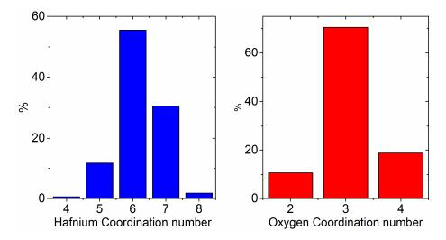
**Figure 10.** Probability distribution of coordination numbers corresponding to the local environments of Hf and O in amorphous HfO<sub>2</sub> nanoparticles.
