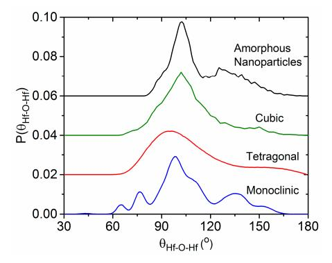
**Figure 11.** Distribution of bond angles monoclinic, tetragonal, and cubic HfO<sub>2</sub> structures obtained from molecular dynamics simulations.
