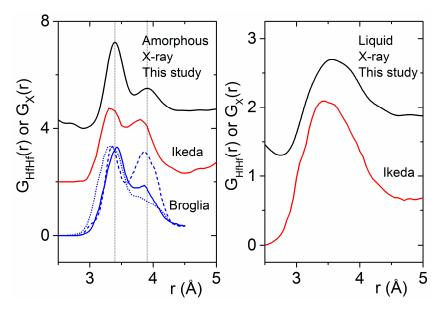
**Figure 8.** (**Left**) Comparison of the experimental X-ray pair distribution functions for amorphous  $HfO_2$  (black) with DFT simulations of the Hf–Hf partial pair distribution function taken from the literature [1,8]. Densities of 8.6, 10.19, and 11.5 g·cm<sup>-3</sup> are denoted by blue dashed, solid, and dotted lines respectively. (**Right**) The same comparison made for liquid  $HfO_2$ .
