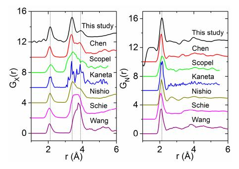
**Figure 7.** Comparison of our experimental pair distribution functions for amorphous HfO<sub>2</sub> (black, top) with several molecular dynamics simulations taken from the literature [2,3,5–7,61] and weighted for: X-rays (**Left**); and neutrons (**Right**).
