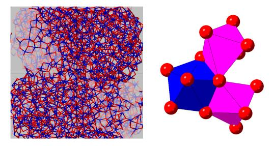
**Figure 12.** Snapshots taken from the MD model of amorphous hafnia nanoparticles: (**Left**) the agglomeration on nanoparticles within the simulation box; and (**Right**) edge- and corner-sharing HfO<sub>n</sub> polyhedra in the low density amorphous form.
