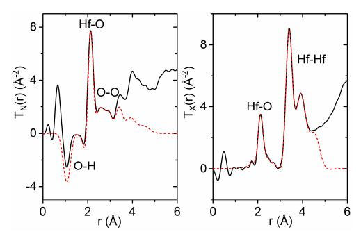
**Figure 3.** Simultaneous Gaussian fits (dashed red) to the measured total pair distribution functions (solid black), assuming a composition of  $(HfO_2)_{0.9} \cdot (H_2O)_{0.1}$ . (**Left**) Total pair distribution function obtained from neutron data,  $T_N(r)$ . (**Right**) Total pair distribution function obtained from X-ray data,  $T_X(r)$ . The negative dips at 1.1 Å and 1.8 Å are assigned to intra-molecular hydrogen bonds in water and O–H groups within the amorphous hafnia network.
