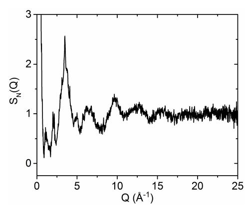
Figure 2. The neutron diffraction structure factor  $S_N(Q)$  measured from the 2010 amorphous hafnia sample.
