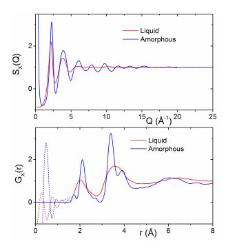
**Figure 5.** (**Top**) Comparison of the X-ray structure factors for liquid HfO<sub>2</sub> and amorphous hafnia nanoparticles. (**Bottom**) A comparison of the corresponding X-ray pair distribution functions  $G_X(r)$ .
