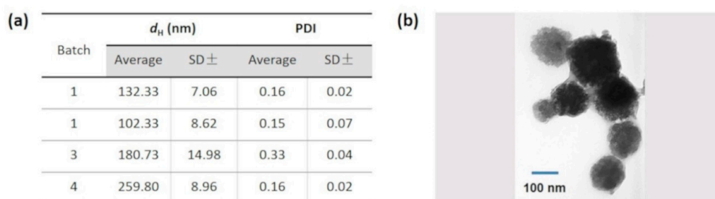
Figure 1. (a) Hydrodynamic diameter, ( d_H , nm \pm SD) and polydispersity index (PDI \pm SD) across the different cocaine nanoMIPs batches obtained by DLS analysis; (b) TEM image (880,000 \times ) of the cocaine nanoMIPs (batch 1).
