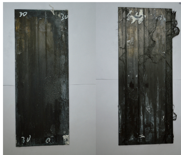
Figure 6. Coated specimen (left side) and naked specimen (right side) immersed in 60 °C alkaline solution for 135 days.
