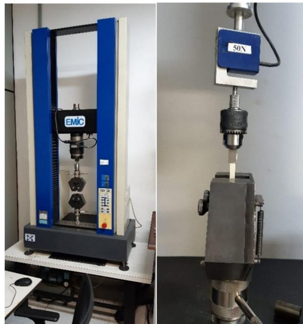
Figure 1. Tensile testing setup.
