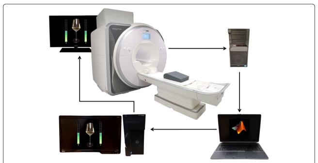
**Fig. 2** rtfMRI Neurofeedback Setup. The scanner computer reconstructs the obtained images and sends them to a laptop with in-house MATLAB scripts for preprocessing and extraction of the neurofeedback signal. The feedback value calculated is then forwarded to a computer with Presentation software and displayed as a thermometer value. The rights to this figure are reserved by the authors
