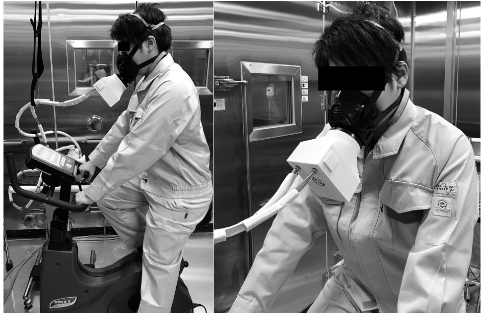
Fig 5. Photograph of the experiment for the measurement of temperature. The subject exercised using the cycle ergometer in a hot artificial climate chamber set at a dry-bulb temperature of 36°C and relative humidity of 45%. The image shows a subject wearing a powered air-purifying respirator equipped with a cooling device.
