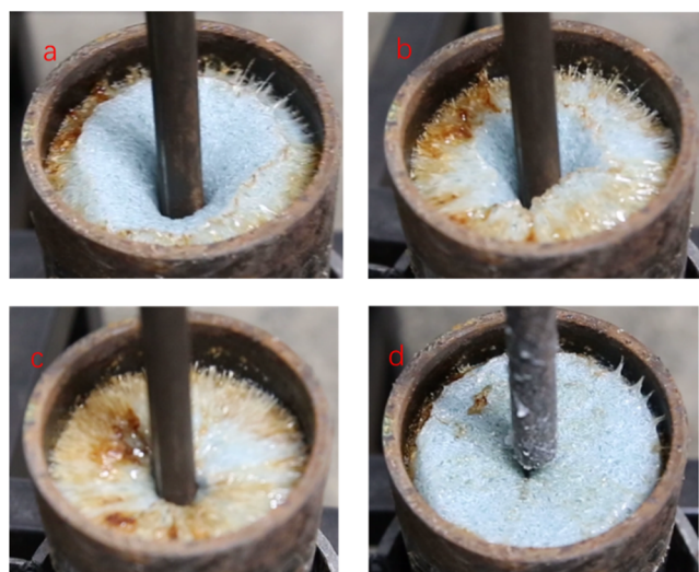
Figure 5. Process of rod penetrating gel slug of sample 4 (Photograph courtesy of Yong Du. Copyright 2023.). (a) Gel was concavely deformed but not broken at the beginning of the penetration. (b) Central area of the gel surface was recessed as the rod moved down. (c) Surrounding colloid moved to the center area. (d) Penetration tunnel shrank after the lifting of the rod.
