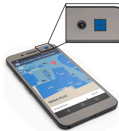
Figure 4. QADA-plus in a typical smartphone. The inset shows the QADA sensor located next to the standard front-facing camera.
