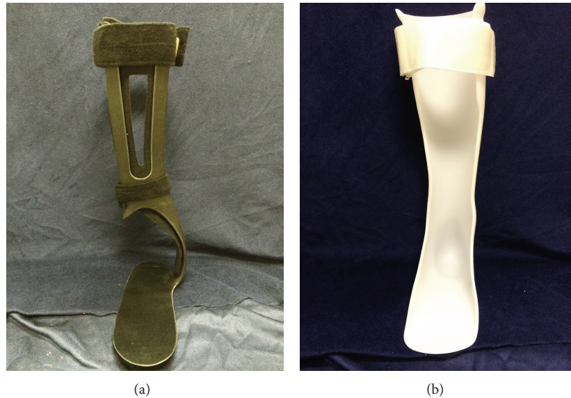
FIGURE 1: Off-the-shelf carbon AFO (a) and custom plastic AFO (b) used in the study.
