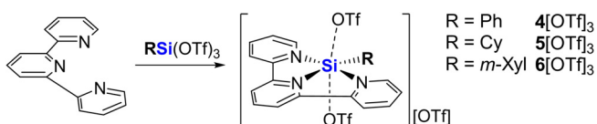
Scheme 2. Synthesis of the triflate salts of trications 4^{3+} , 5^{3+} and 6^{3+} .
