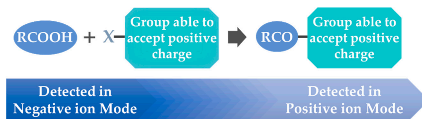
Figure 3. Basic principle of FA derivatization for its charge reversal.
