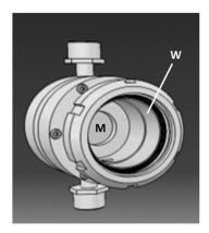
**Figure 5.** Membrane module especially designed for coupling photocatalysis and membrane filtration. (**M**) flat membrane; (**W**) window in borosilicate glass transparent to near-UV light.
