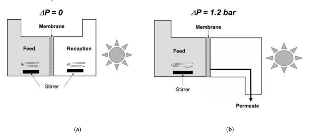
**Figure 3.** Schematic representations of cells used for assessing the functional performance of membranes photocatalytically functionalized on the permeate side. (a) Diffusion set-up and (b) permeation set-up.
