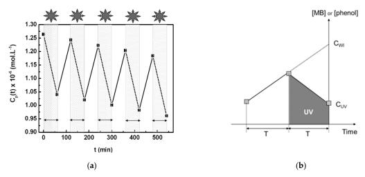
**Figure 4.** Measurement of the parameter  $\delta$  equal to the quantity of organic solute photodegraded per units of time and of membrane surface area. (a) Concentration of Methylene Blue (MB) in the reception compartment with alternate periods with or without UV irradiation, using the macroporous disk with grains coated by mesostructured anatase. (b) Graphical representation of the method used for calculating  $\delta$ .
