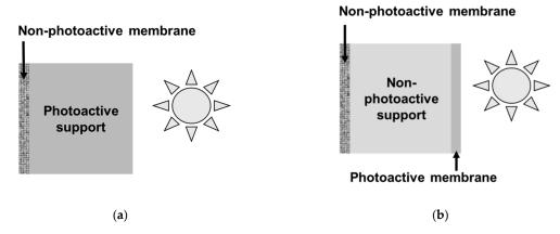
**Figure 1.** Photocatalytic membranes with ultraviolet (UV) irradiation on the permeate side; (a) intrinsically photoactive substrate, and (b) covering of the substrate grains with a photocatalytic coating or photoactive film deposited on the porous substrate.
