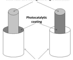
Porous ceramic hollow fiber as a separative membrane
