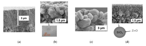
**Figure 2.** Cross section images obtained by a scanning electron microscope. (a) Anatase film from a commercial titania hydrosol, (b) coating on substrate grains from a nanocrystalline titania sol, and, as an insert, a transmission electron microscope image showing the ordered mesoporosity of the coating, (c) PECVD titania coating on substrate grains, and (d) mesoporous film of SiO<sub>2</sub>/ZnO nanoparticles.
