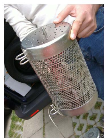
One passive sampler (Figure 4), a semi-permeable membrane device (SPMD), was placed at each site for one month in spring (May 7–June 4) and autumn (September 17–October 15). Semi-permeable membrane device sampler consists of a horizontal thin-walled tub from nonporous low density polyethylene, filled with synthetic lipid (triolein). The SPMD were commercially manufactured (Exposmeter AB, Sweden). After exposure the sampler membranes were rinsed briefly
