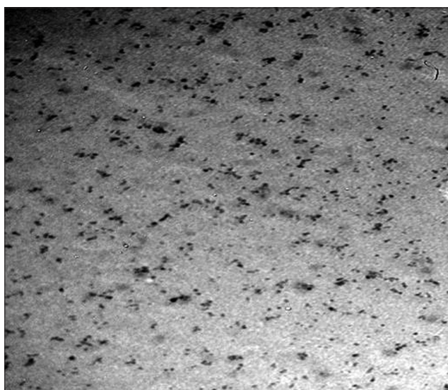
Figure-4: TEM image for propolis nanoemulsion (PNE) showed the PNE with average size of 36.66 nm.
