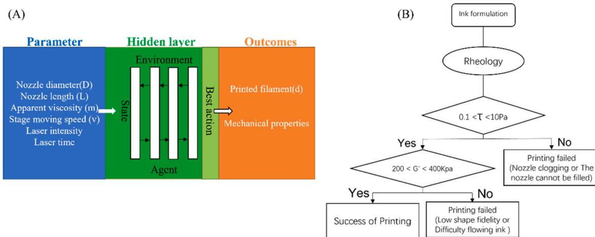
**Fig. 7.** Example of a 3D printed organ model applying a neural network. (A) The printing parameters are fed into the neural network as training data to predict the filament diameter and the mechanical properties of the material. (B) Development of flowcharts for ink. Modified with permission from Ref. [94]. Copyright 2022 MDPI.
