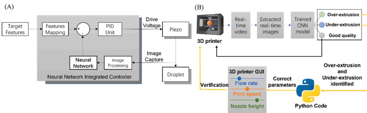
**Fig. 8.** Example of Closed-Loop AI Printing. (A) Closed-loop voltage control framework for the Liquid Metal Jet Printing process. Reproduced with permission from Ref. [107]. Copyright 2018 Elsevier. (B) Workflow of a closed-loop feedback control algorithm based on a convolutional neural network (CNN) model. Modified with permission from Ref. [108]. Copyright 2019 Elsevier.
