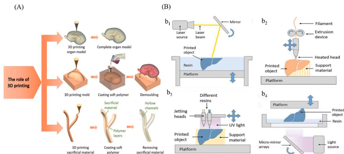
**Fig. 2.** Schematic diagram of the different types of direct and indirect printing and direct printing. (A) Direct 3D printing of organ models, 3D printing of casting molds, and 3D printing of sacrificial material fabrication models. (B) b<sub>1</sub> Stereo lithography Appearance (SLA), b<sub>2</sub> Fused Deposition Molding (FDM) , b<sub>3</sub> Inkjet printing, b<sub>4</sub> Digital Light Processing (DLP). Reproduced with permission from Ref. [13]. Copyright 2021 Wiley.
