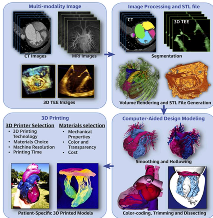
**Fig. 3.** The process of 3D printing organ models. Take 3D printing heart models as an example. Reproduced with permission from Ref. [27]. Copyright 2021 Elsevier.
