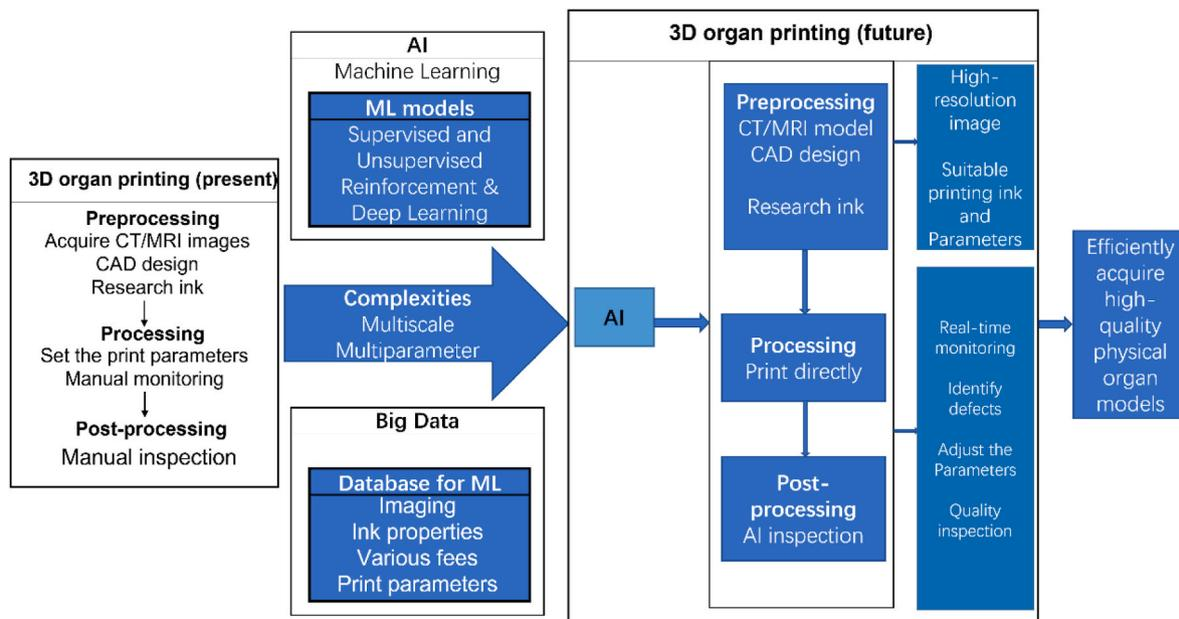
Fig. 9. Future perspectives on the use of AI for 3D printing of organ models. Modified with permission from Ref. [24]. Copyright 2021 PubMed Central.
