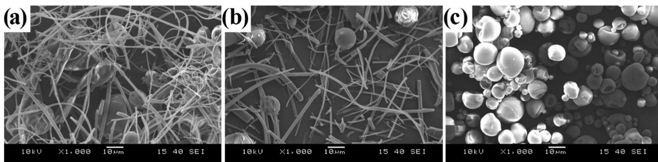
Figure 3. SEM images of the ES before grinding (a), after grinding (b), and the SD (c) samples.
