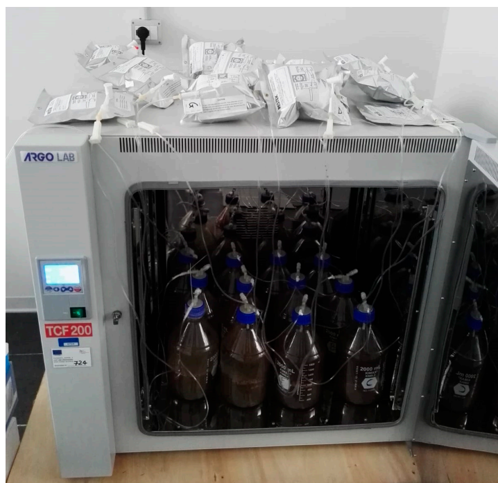
Figure 2. Biochemical methane potential (BMP) tests of olive mill wastewater under mesophilic conditions (37 °C). Source: Picture acquired in our own laboratory.
