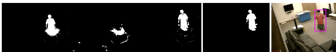
Figure 4. Human extraction result. First frame correspond to the Codebook result, the second one is the shadow detection. with simple subtraction between CB result and shadow detection, we get the third frame. After applying the second step from post processing, we get the result in the fourth frame. The last frame illustrates the tracked object correspond to the human silhouette.
