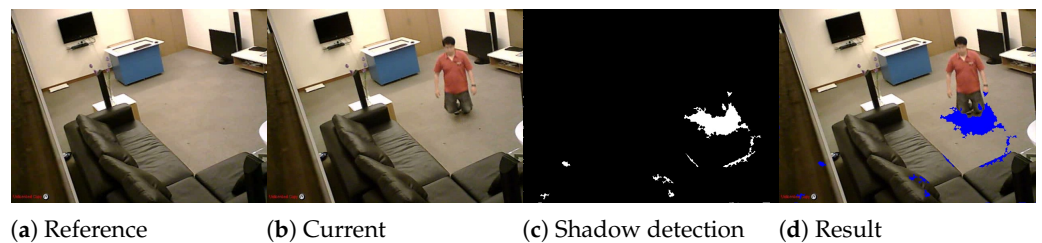
Figure 3. Illustration of Shadow detection. (a) The reference frame. (b) The current frame. (c) Shows the detected shadow pixels in current frame. (d) the result of shadow detection showed with blue color in current frame.
