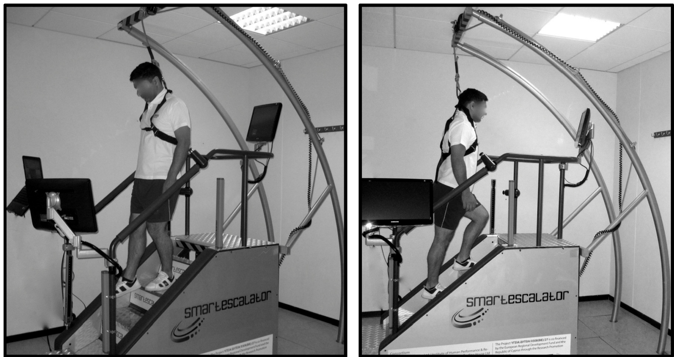
Figure 1. The automatic escalator device was invented, designed and constructed by our group and it is the first of its kind offering both stair descending (eccentric-biased) and stair ascending (concentric-biased) exercise.
