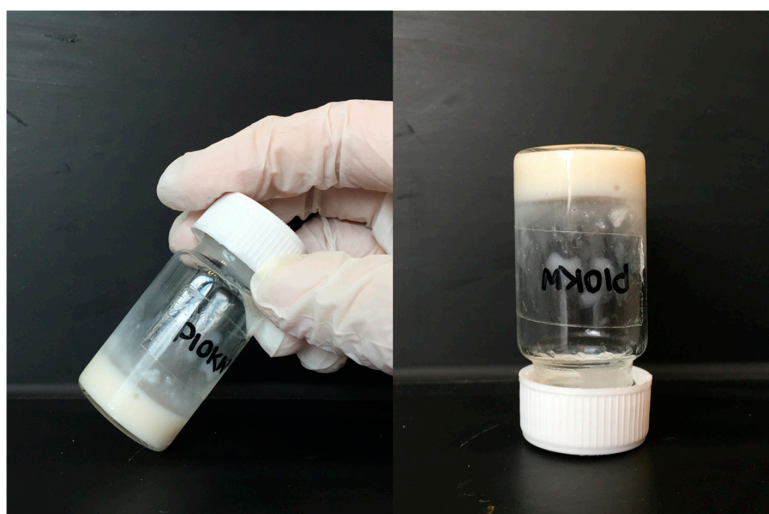
Figure 2. The preparation of pectin-PEGMA/ \alpha -CD gels.
