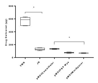
**Figure 6.** Aerosol drug delivery using LTV ventilation during simulated mechanical ventilation with active humidification. Three different devices, VMN, JN, and pMDI, using three different spacer/adapter types, were tested. pMDI actuation was at the start of inhalation. Results are presented as mean  $\pm$  SD  $\mu$ g drug delivered. \* Denotes statistical significance at p < 0.0001.
