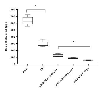
**Figure 4.** Aerosol drug delivery using standard adult settings during simulated mechanical ventilation with active humidification. Three different devices, VMN, JN and pMDI, using three different spacer/adapter types, were tested. pMDI actuation was at the start of inhalation. Results are presented as mean  $\pm$  SD µg drug delivered. \* Denotes statistical significance at p < 0.0001.
