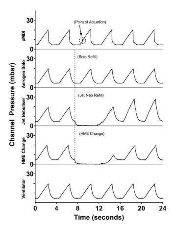
**Figure 7.** Ventilator circuit pressure change during nebuliser drug refill, pMDI actuation and HME change. Testing was completed using a pressure sensor. Results are presented as circuit pressure in mbar over time in seconds.
