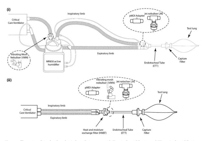
$\textbf{Figure 2.} \ \ \textbf{Illustration of simulated mechanical ventilation setup with (i) active humidification and (ii) passive humidification.}$
