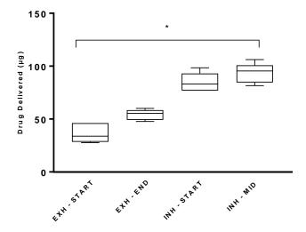
**Figure 3.** Drug delivery from pMDI actuation at different stages of the respiratory cycle (INH = inhalation; EXH = exhalation) during simulated mechanical ventilation with active humidification. Testing was completed with the pMDI and the MiniSpacer. Results are presented as mean  $\pm$  SD  $\mu$ g drug delivered. \* Denotes statistical significance at p < 0.0001.
