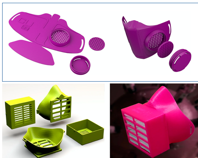
Figure 5. 3D-printed protective face mask. Reprinted with permission from ref 22. Copyright 2020 John Wiley & Sons.
