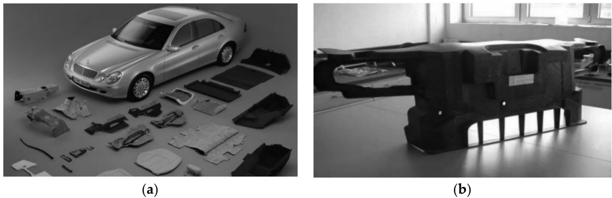
Figure 6. Natural composites applied in the automotive sector (a) Components of Mercedes-Benz E-Class (b) Ford Montageträger front-end grill (available under a Creative Commons license [26]).
