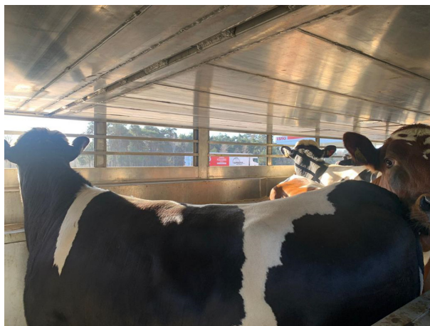
Figure 8: Heifers during transport with their heads significantly above the height of the withers – illustrating the need for sufficient vertical space during transport. Photo by Lars Kloster, VikingDenmark, taken inside a two-deck cattle truck
