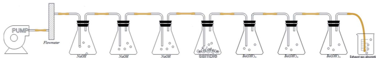
Fig. 1 Device used to detect the amount of CO 2 evolved by PLA/PHB-blended nonwovens during the degradation process.
