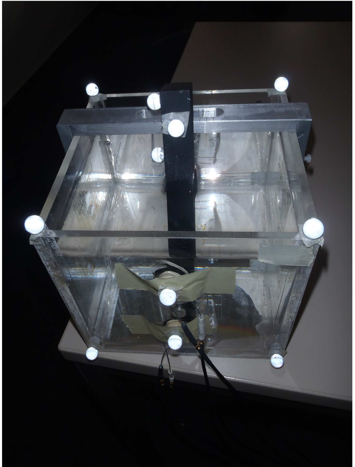
Fig 6. A rod rotated in a water bath with reflective markers.
