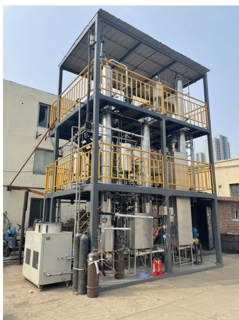
Fig. 7 | The physical picture of the pilot plant for continuous C4 gas mixture sorption-desorption separation experiment. The main body of the equipment is two packed columns, which are used as absorption column and desorption column respectively, with a height of about 5.5 m.
