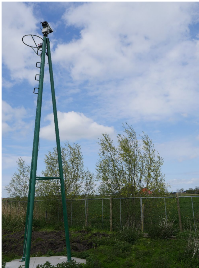
Figure 3. The laser placed on a steel, three-legged tower (the top was 6 m above ground level) that was secured to a concrete slab (1.5 m × 1.5 m) weighing approximately 2000 kg (source: photo by first author).
