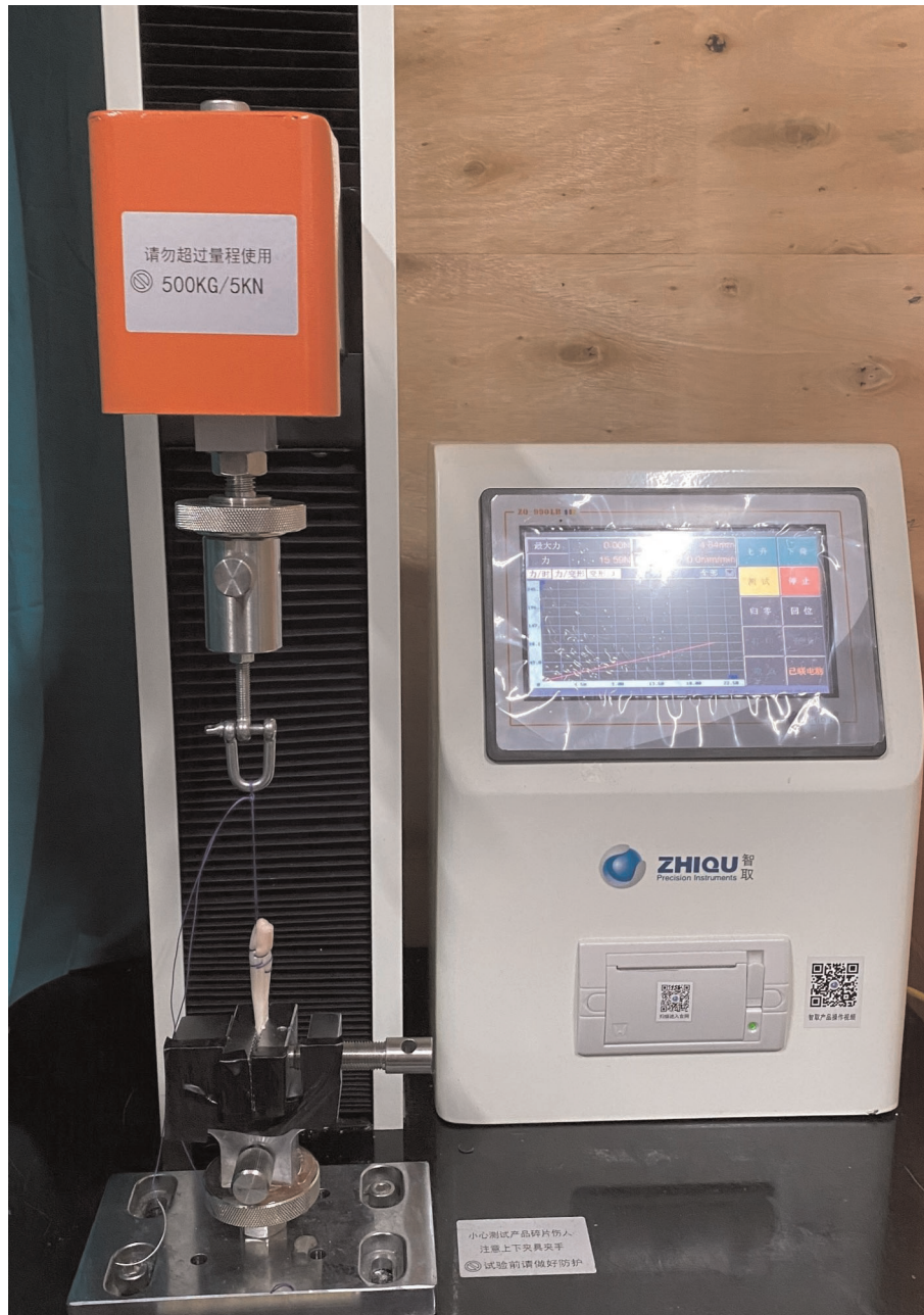
FIGURE 2 | The graft with the needle stitching technique is placed in an electric tensile test system before the pretension test.
