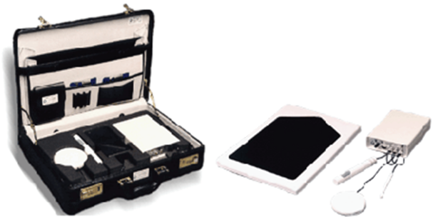
FIGURE 1: The Coordination Ability Test System (CATSYS) including a data logger and four different sensors: a tremor pen, a touch recording plate, a reaction time handle, and a force plate for balance (static posturography) recording.
