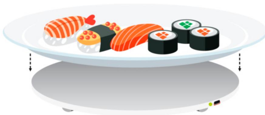
**Figure 5.** A custom-made electronic scale that is connected via bluetooth with a smartphone application measuring the reduction of the food placed on the scale along with self-recording of hunger and fullness [54].
