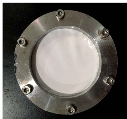
Fig. 2 Custom holder assembled with an PES substrate layer for PDMS coating.
