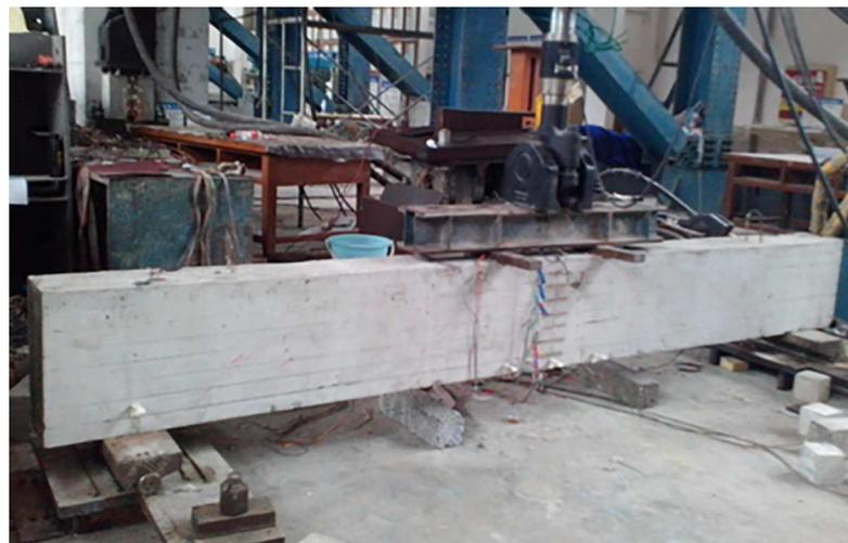
**Fig 5. Fatigue test loading site.**
