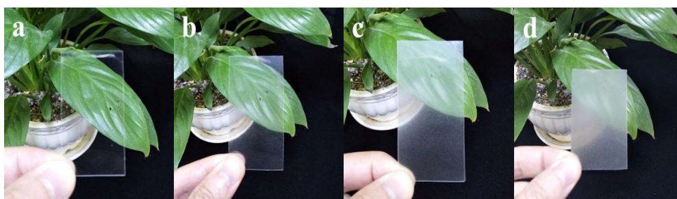
Figure 3. Visual images of PLA/CNF biocomposite films: (a) neat PLA; (b) PLA/CNF-1.0 wt %; (c) PLA/CNF-2.5 wt %; and (d) PLA/CNF-5.0 wt %.
