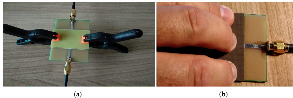
Figure 7. Measurements on FR4 with clamps and TLX8 with fingers. (a) measurement of FR4. (b) measurement of TLX8.
