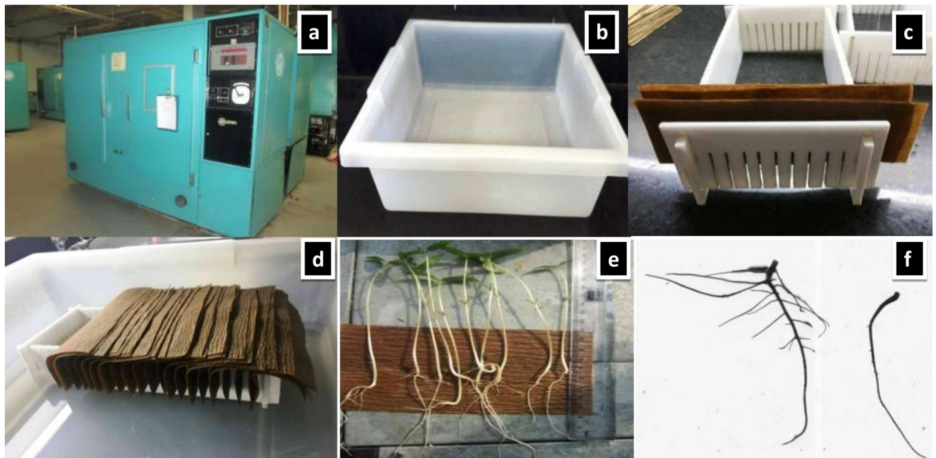
Fig 1. Semi-hydroponic phenotyping platform (a) growth chamber (b) plastic tray (c) germination stand and paper setup (d) germinating mungbean seeds in semi-hydroponic phenotyping platform (e) seedling grown for 18 days (f) root system of two contrasting genotypes grown for 18 days.
