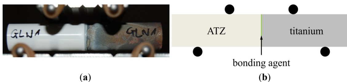
Figure 2. Four-point-bending test setup for a soldered compound sample (a); shown schematically (b); indicating supports on the bottom and loading noses on the top (black circles).
