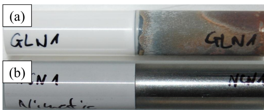
Figure 1. Compound samples after glass soldering (a) and adhesive gluing (b) of the ceramic and titanium components.
