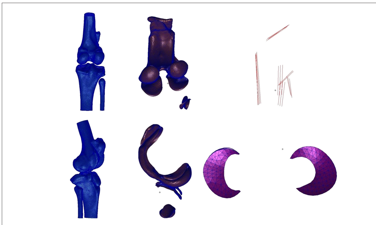
Figure 7. Finite element mesh model of the sheep knee joints in posterior and lateral views, showing the bone ( left ), articular cartilage ( middle ), and peripheral ligament and meniscus ( right ).
