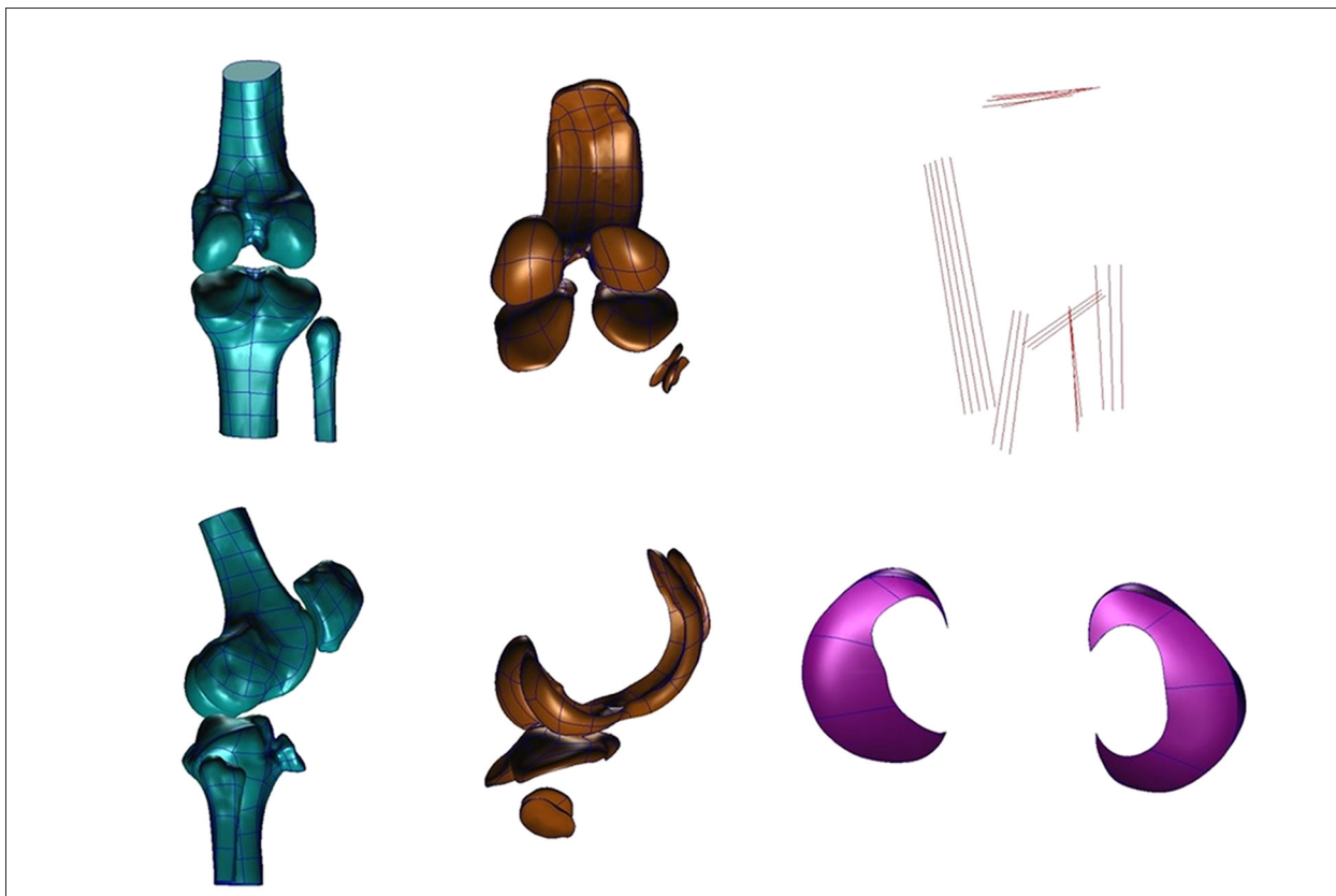
Figure 1. Geometric model of the mini-pig knee in posterior ( top ) and lateral ( bottom ) views, showing the bone ( left ), articular cartilage ( middle ), and peripheral ligament and meniscus ( right ).
