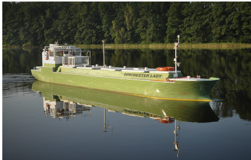
Figure 1. “Dorchester Lady” training ship—scale model of 113,500 Deadweight Tonnage (DWT) Liquefied Natural Gas (LNG) carrier.
