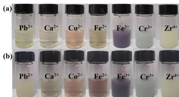
Figure 2. Sample vials containing DMF (1 mL) solution of amPEN (50 mg) added with different metal ions aqueous solution ( 10^{-2} M) after stirring for 10 min (a) and 24 h (b).
