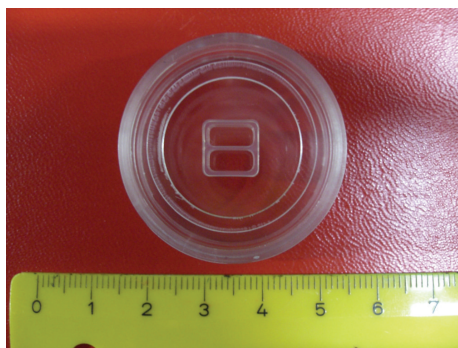
FIGURE 1: Culture-insert in a 24-well format dish to produce uniform scratches in parallel samples.
