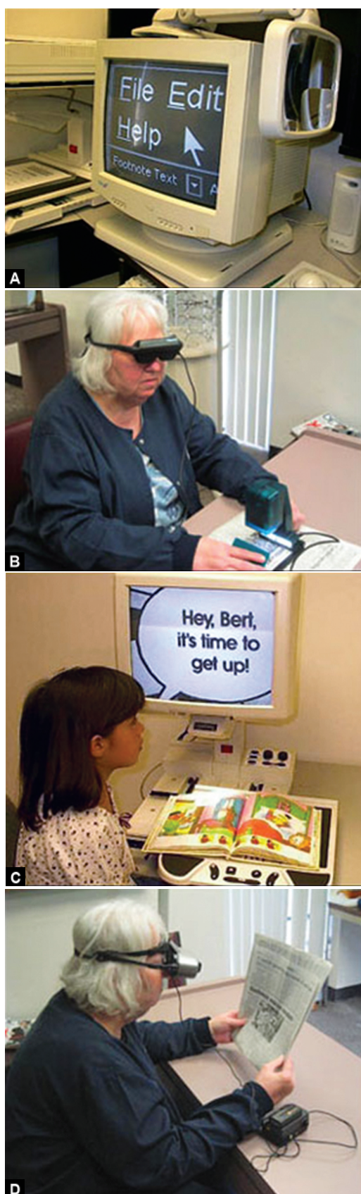
Figs 4A to D: (A) Computer magnification software, (B) patient using a hand-held camera, (C) patient using a CCTV, (D) patient using a head-mounted camera (source: www.lowvision.org )
