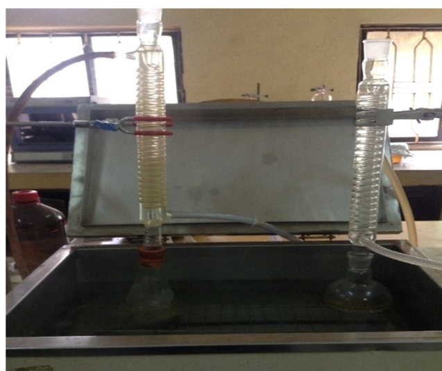
Figure 3. Epoxidation (3 h at 60 °C)/hydroxylation reaction (3 h at 60 °C then 14 h at 80 °C).
