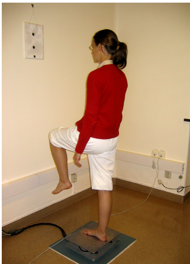
Figure 1 Stabilometry in single-limb stance, tested by means of a strain gauge force plate. A standardized position was used. The subject is a model who did not participate in the study.
