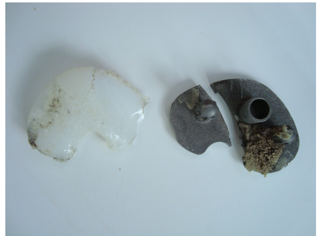
Fig. 3. Intraoperative view of the fractured tibial component (A) and the fractured tibial component showing bone ingrowth in the lateral part of the knee with severe polyethylene wear (B).
