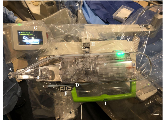
Figure 3 Corpath GRX robotic arm and cassette (Corindus). This is one of two commercial systems to have been used for neurointervention. A. Sheath attachment. B. Guide catheter rotation module. C. Guide support track. D. Rapid exchange device port. E. Guidewire rotation module. F. Micro-adjustment buttons. G. Robotic arm feedback console. H. Cassette locking mechanism. I. Robotic arm toggle button. Reproduced with permission from BMJ Publishing Group Ltd. 18
