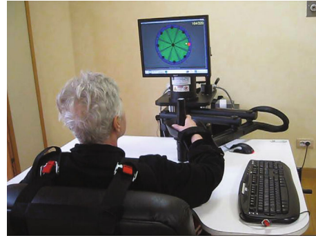
FIGURE 1: Upper limb RT based on the InMotion 2.0 robotic system.
